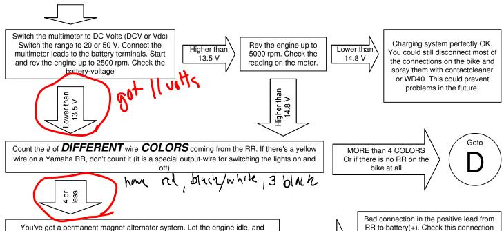
You've got a permanent magnet alternator system. Let the engine idle, and connect the black multimeter-lead up to the battery(+). Connect the RED multimeter lead up to the RED (or WHITE/RED = Kawasaki) output wire of the RR. Leave the RR connected up to the bike. Check the reading on the meter.
