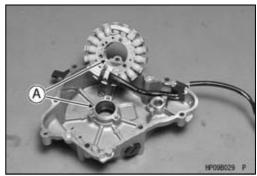
• Apply silicone sealant to the circumference of the stator coil lead grommet, and fit the grommet into the notch of the cover securely.
