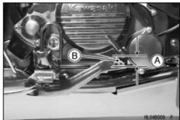
Rear (Parking) Brake Lever and Pedal Free Play Adjustment
