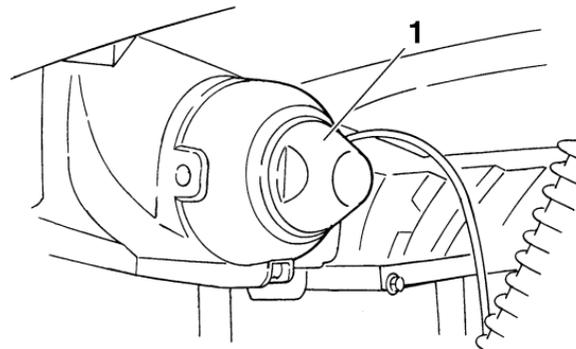
2. Remove the headlight bulb holder cover by pulling it off.
