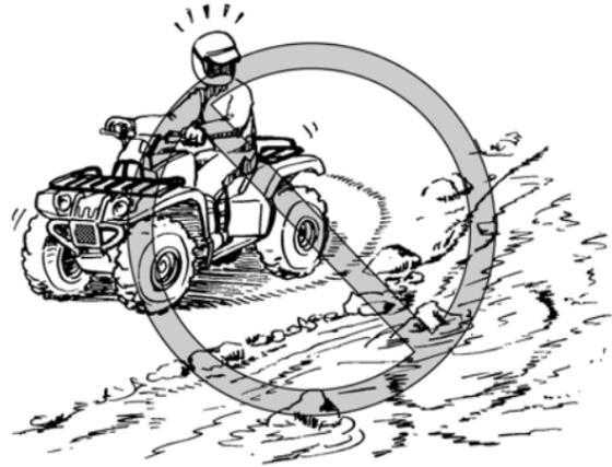
Test your brakes after leaving the water. Do not continue to ride your ATV without verifying that you have regained proper braking ability.
