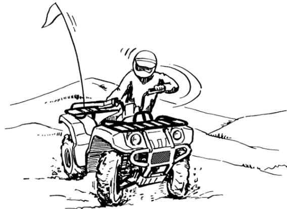
If the rear wheels of your ATV start to slide sideways, control can usually be regained (if there is room to do so) by steering in the direction of the slide. Applying the brakes or accelerating is not recommended until you have corrected the slide.
