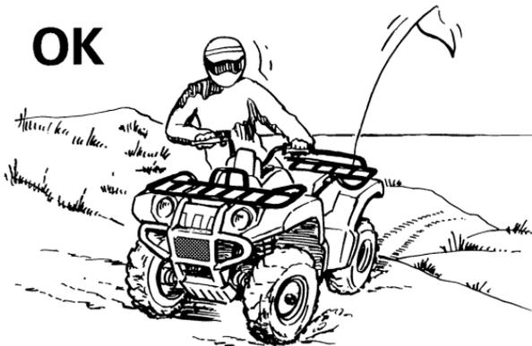
If your ATV has stalled or stopped and you believe you can continue up the hill, restart carefully to make sure you do not lift the front wheels which could cause you to lose control. If you are unable to continue up the hill, dismount the ATV on the uphill side. Physically turn the ATV around and then descend the hill.
