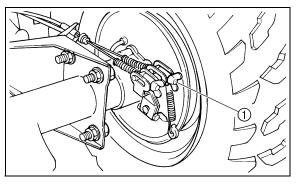
1. Adjusting nut (brake rod)
