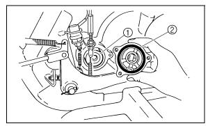
1. Engine oil filter element
