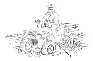
Your Sportsman 6X6 can operate through water with a maximum recommended depth equal to the footrests (1). Avoid operating the ATV through deep or fast-flowing water. If you cannot avoid water that exceeds the recommended maximum depth, go slowly, balance your weight carefully, avoid sudden movements, and maintain a slow and steady forward motion. Do not make sudden turns or stops, and do not make sudden throttle changes.
