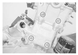
• Install the cam chain tensioner.
