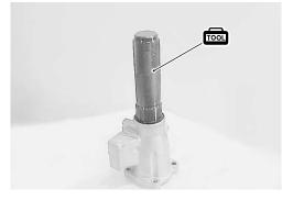
Apply grease to the seal lip groove.
