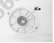
Apply a small quantity of SUZUKI MOLY PASTE to the armature shaft.
