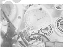
Measure the backlash by turning the drive bevel gear shaft in each direction, reading the total backlash on the dial gauge. If the backlash is not within specification, the shim must be changed and the backlash should be re-checked until correct. Refer to the chart at the right for appropriate shim thickness.
