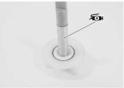
• Install the E-ring to the impeller shaft.
