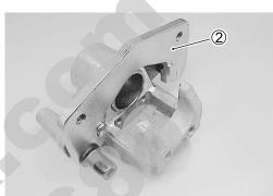
• Place a rag over the brake caliper pistons to prevent them from popping out and then force out the pistons using compressed air.
