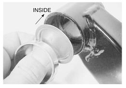
• Apply SUZUKI SUPER GREASE "A" to the swingarm bearings and lips of dust seals, then install them into the swingarm with the special tool.
