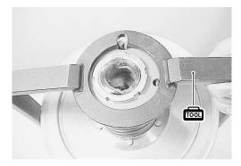
• Install the spring and spring plate by aligning the spring ends with the holes.
