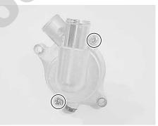
Install the water pump and tighten its mounting bolts to the specified torque.
