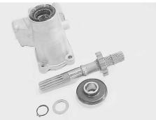
• Remove the parking gear by removing the snap rings.
