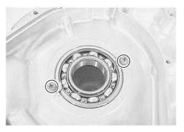
• Remove the bearing with the special tool. 09913-70210: Bearing installer/remover set тоо • Remove the oil seal with the special tool. 09913-70210: Bearing installer/remover set REASSEMBLY • Install the oil seal with the special tool. 09913-70210: Bearing installer set • Install the bearing with the special tool. 09913-70210: Bearing installer set · When installing the bearing retainers, apply a small quantity of THREAD LOCK to the screws. **€**1342 09900-32050: THREAD LOCK "1342"
