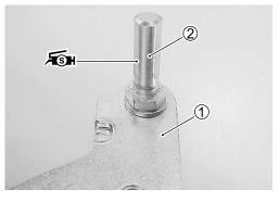
• Apply THREAD LOCK SUPER "1360" to the nut ③ and tighten it to specified torque.
