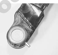
• Remove the knuckle end by using the special tools.
