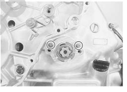
• Install the new gaskets ④ and tighten the speed sensor mounting bolts.
