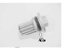
• Apply sealant to the 2WD/4WD switches and tighten them to the specified torque.
