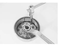
• Install the starter clutch in the proper direction.
