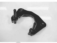
Apply SUZUKI SILICON GREASE to the brake caliper holder pins.
