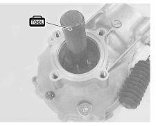
• Remove the bearing from the shaft with a commercially available bearing puller or hydraulic press.
