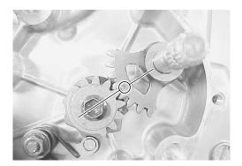
• Reassemble the gearshift shaft.
