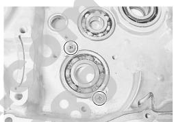
• Remove the bearing with the special tool.
