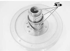
• Install the rollers and pins.
