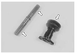
Inspect the parking cam, thrust bearing and return spring for any flaws or damage. If any defects are found, replace the cam, bering and spring with the new ones.
