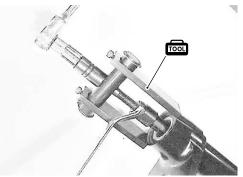
• Remove the hub bearings using the special tool.
