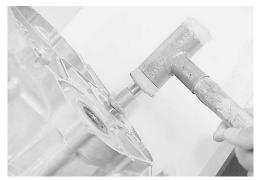
• Remove the output shaft with a plastic mallet.
