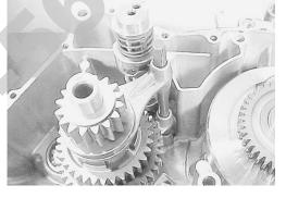
• Install the transfer input shaft ①.
