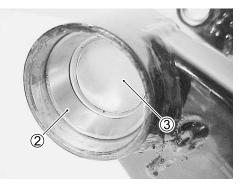
• Remove the swingarm bearing race and bearing plate by using the special tool.
