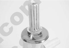
• Remove the drive shaft and waterproof seal by tapping with a plastic mallet.
