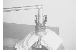
Remove the washer ①, joint yoke ②, oil seal ③ and bearing ④.
