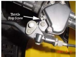
the throttle travel thus reducing the maximum speed of the unit. Turning the stop screw counter clockwise will increase the throttle travel thus increasing the maximum speed of the unit. Tighten the stop screw locking nut when the desired throttle travel has been established.
