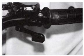
The throttle lever is located on the right-hand handle bar below the grip. To operate the throttle lever, place your right thumb on the lever and press forward to increase your speed. To decrease your speed, reduce your pressure on the lever and the spring tension will automatically reduce your speed.
