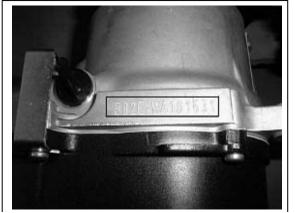
Engine serial number is located on the left-hand side of the engine on the crankcase housing.
