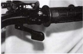
The throttle lever is located beside the righthandlebar grip and is operated by using the righthand thumb. The lever is spring loaded and will return to the idle position when you remove your thumb from the lever. To accelerate the unit, simply press the lever forward to open the throttle slide in the carburetor. To slow the unit, reduce the pressure on the lever or remove your thumb and the throttle will return to the idle position automatically.
