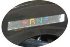
The selector **must be placed on "N"** to start the engine. Once the engine is started, engine the brake lever and move the selector switch to the desired direction of travel.
