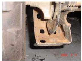
After riding your unit, be sure to clean any build up of mud, sand and dirt from the brake rotor skid plate. This will protect the rotor disc from rust and corrosion.
