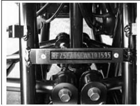
Vehicle Identification Number (VIN) is located at the front of the unit under the front fender on a plate mounted between the main frame rails.
