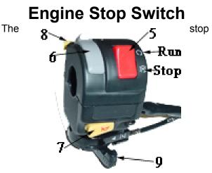
switch is a red colored rocker switch located on the left-hand handle bar.
