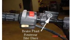
or leaks. Check the fluid level in the fluid reservoir by checking the site glass for the level.
