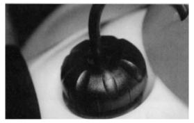
unit just ahead of the seat. The cap contains a vent to prevent a vacuum from forming in the tank as fuel is used. The vent tube must be attached to the cap and inserted in the vent tube holder hole while operating the unit. The fuel cap vent and vent tube must be clean and clear of obstructions for the unit to operate normally. You can check the vent and vent tube by blowing air through the tube. If you can not blow through the vent tube and cap you must clean the vent and tube or replace them.
