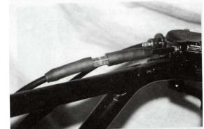
travel before the throttle engages the carburetor throttle slide. To adjust the cable's free travel, loosen the locking nut of the cable adjuster, and turn the adjuster wheel until there is 1/8" free travel in the lever. Tighten the locking nut to secure the adjusting ring.
