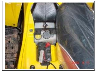
Your ATV uses 2 cycle oil to lubricate the engine. The oil tank is located under the seat at the front of the unit. Oil is drawn from this tank by an oil injector pump when the engine is operating.
