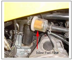
Check the filter for dirt or damage before each ride and at each refueling. Replace the filter if dirty or damaged.
