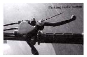
This feature must be engaged in order to start the engine. The brake lever has a safety switch built in to prevent the engine from starting while the brake is disengaged. If your engine fails to start, ensure that the engine stop switch is in the on, "**O**", position and that the parking brake is engaged.
