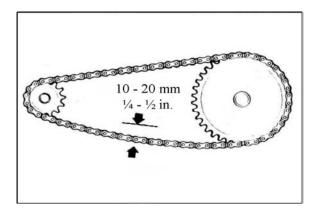
The amount of slack in the chain should not exceed 10-20mm or  $\frac{1}{4}$ " -  $\frac{1}{2}$ ".
