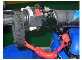
The Viper 50M and Viper 70 models are equipped with a safety tether switch (optional on Viper 90R). The switch is located on the left hand side of the handlebars. The switch cap must be fully engaged for the vehicle to start and run.
