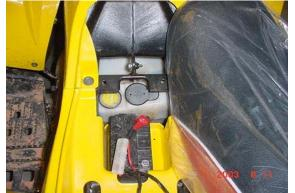
supplies electrical power to the unit. The battery is a 12 volt jell acid type that contains no liquid electrolyte. The battery should be removed from the vehicle when stored for extended periods and charged before being replaced in the unit. Use a trickle charger set at 12 volts to recharge the battery to full charge before replacing it in the unit.
