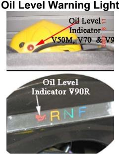
The unit is also equipped with an oil level indicator lamp. The lamp will light when the oil level in the tank is low. When the lamp is lit you MUST refill the oil tank.
