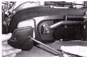
This unit is equipped with an air filter for the C.V.T. transmission. It is located on the lefthand side of the engine, just ahead of the kick starter spindle. The filter will accumulate dust and must be cleaned periodically to maintain normal vehicle operations. Inspect and clean the filter every 30 operating days, more frequently if operated in a dusty environment.
