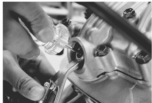
Apply grease to new O-rings and install them to the valve inspection caps.
