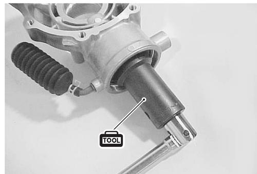
Remove the pinion gear assembly and shim.
