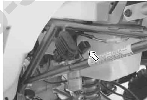
First check the insulation between Ⓐ and Ⓑ terminals with the tester. Then apply 12 V to terminals as shown and check the continuity between Ⓐ and Ⓑ. If there is no continuity, replace the neutral relay with a new one.
