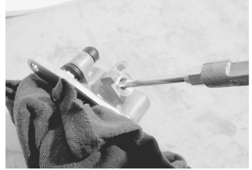
Remove the dust seal and piston seal.
