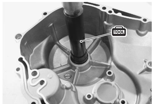
Install the clutch release outer guide ①.
