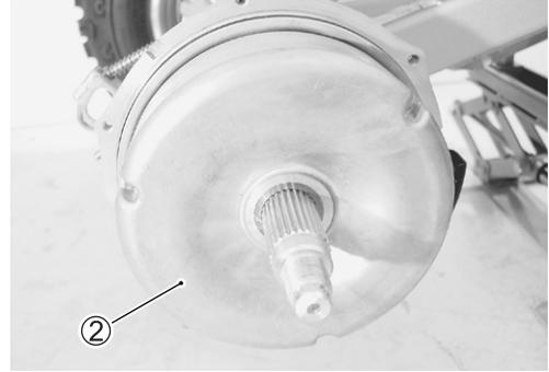
Install the drum cover and tighten the bolts.
