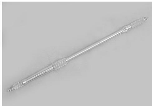
Using a dial gauge, check the axle shaft for runout and replace it if the runout exceeds the limit.
