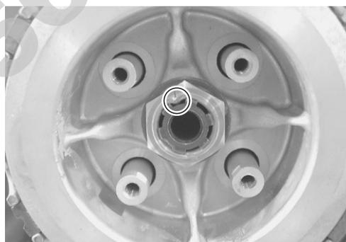
Remove the clutch sleeve hub nut with the special tool.
