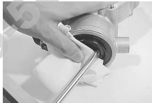
Unstake the bearing locknut with a small chisel or drill.
