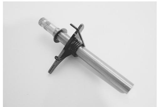
Install the shift cam lock shaft by fitting the spring end to the stopper properly.
