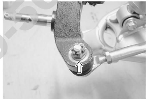
Disconnect the tie rod end with a commercially available ball bearing joint remover ④.
