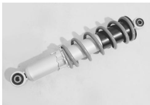
Inspect the rubber bushing for wear or damage.
