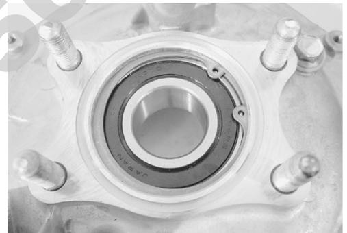
Install new dust seal ② to the drum cover ③ by using the removed dust seal ①.
