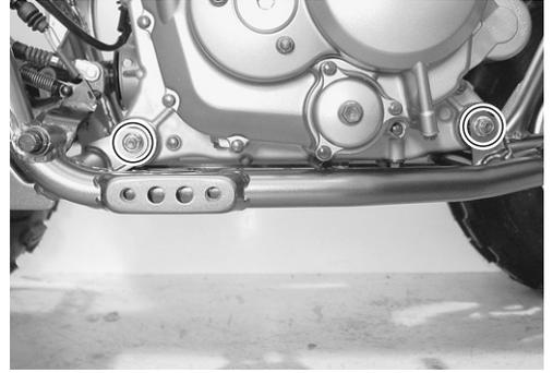
Disengage the secondary driven gear shaft from the universal joint.
