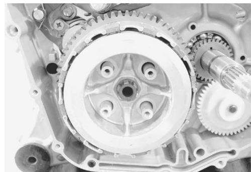
Install the washer and clutch sleeve hub nut.
