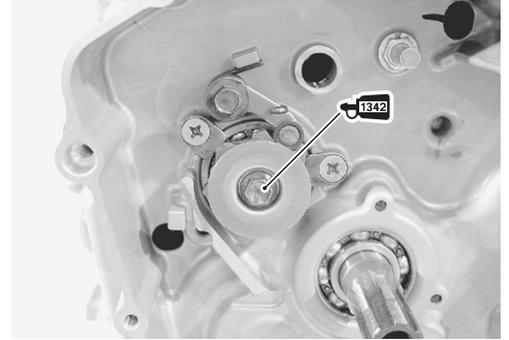
Install the gearshift cam shaft assembly so that the stopper **⑤** comes between the spring ends **⑥**.
