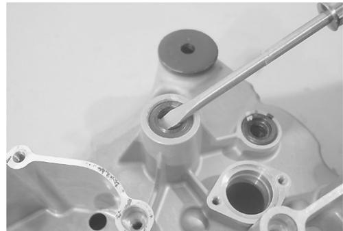
Apply SUZUKI SUPER GREASE to the oil seal.
