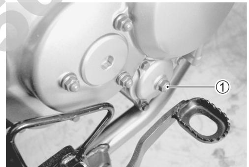
Install the oil pressure gauge and adaptor into the main oil gallery.
