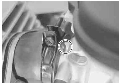
Position the carburetor clamps as shown in the illustration. Connect the carburetor hoses properly. (➔9-16)
