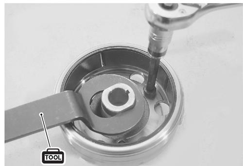
Install the starter clutch in the proper direction.
