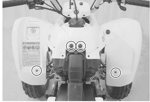
Open the fuel tank cap and remove the fuel tank top cover ①.
