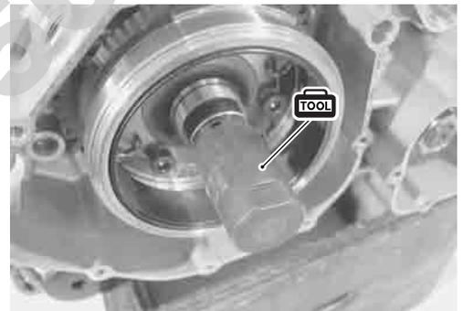
Remove the generator rotor with the special tool.
