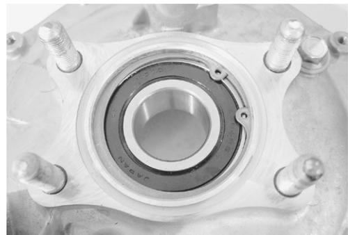
Remove the bearing with the special tool.
