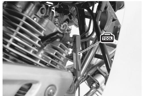
Start the engine and set the engine idle speed between 1 400 and 1 600 r/min by turning the throttle stop screw knob  $\text{\textcircled{1}}$ .
