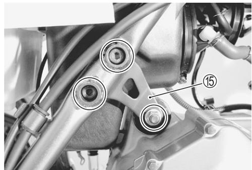
Remove the front and rear lower engine mounting nuts and bolts.
