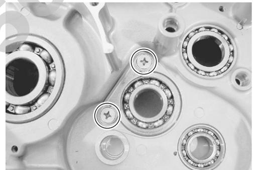
Remove the bearings with the special tools.
