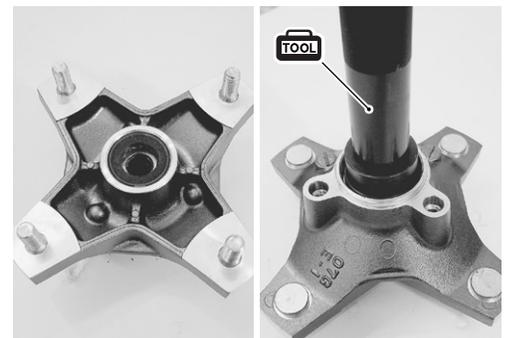
Install the spacer ④ to the front wheel hub.
