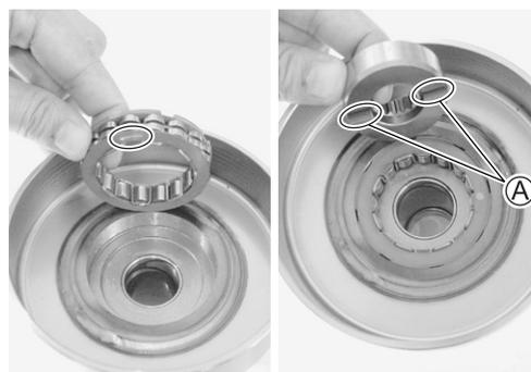
Install the clutch wheel assembly.
