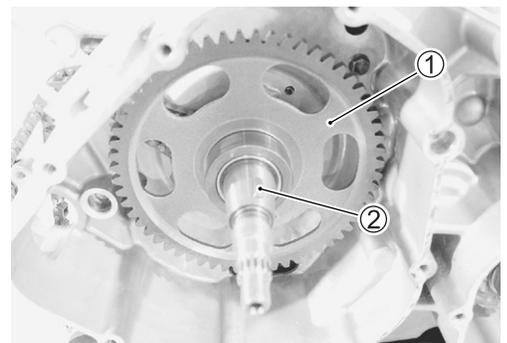
Install the generator rotor and tighten the generator rotor nut to the specified torque with the special tool.
