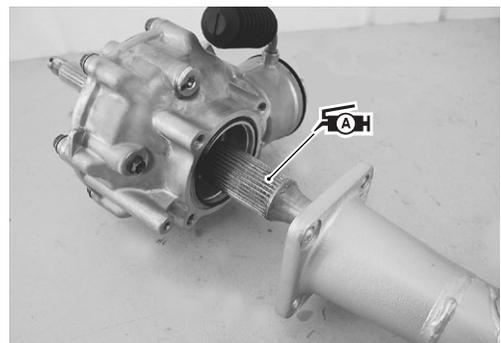
Apply THREAD LOCK SUPER to the axle housing/final gear case bolts, and tighten them to the specified torque.
