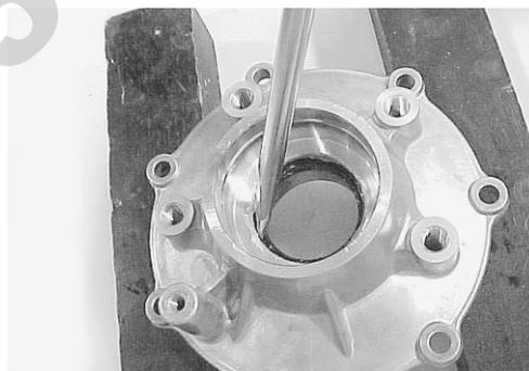
Remove the oil seal with a suitable tool.
