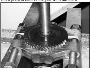
23. Make note of the direction of the gear and hub location.
