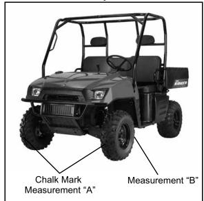
NOTE: It is important that the height of both marks be equally positioned in order to get an accurate measurement.
