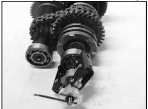
16. Remove the park lock engagement dog. Remove the wave spring and reverse engagement dog.
