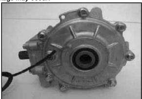
Cover Bolts Torque: 17 ft. lbs. (23 Nm)
