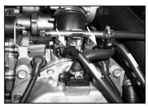
When the key switch is on, the fuel rail is pressurized, and voltage is present at the injector. At the proper instant, the ECU completes the ground circuit, energizing the injector. The valve needle in the injector is opened electromagnetically, and the pressure in the fuel rail forces fuel down through the inside. The "director plate" at the tip of the injector (see inset) contains a series of calibrated openings which directs the fuel into the intake port in a cone-shaped spray pattern.
