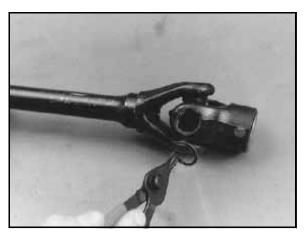
NOTE: If yoke or bearing is removed, cross bearing must be replaced. Note orientation of grease fitting and mark inner and outer yoke for correct repositioning during installation.
