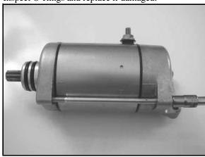
NOTE: Note the alignment marks on both ends of the starter motor casing. These marks must align during reassembly.
