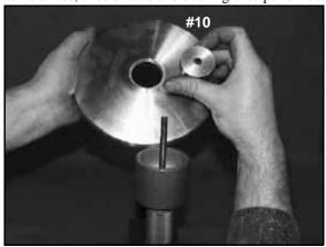
5. Install the nut removed in Step 2 onto end of puller rod and hand tighten. Turn puller barrel to increase tension on sheave if needed. Nut is left hand thread
