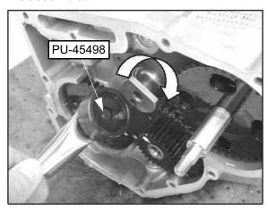
27. Reinstall the camshaft gear; so the timing marks are properly aligned. Install the washer and bolt. Torque to specification.
