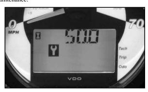
NOTE: The service interval is programmed at 50 hours at the factory.
