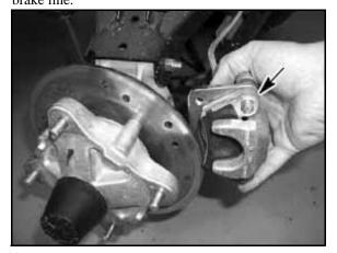
5. Remove hub cap, cotter pin, front spindle nut, and washer.
