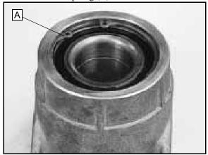
2. From the back side, tap on the outer bearing race with a drift punch in the reliefs as shown in Figure 7.24.
