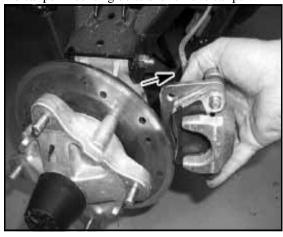
4. Clean disc, caliper body, and pistons with brake cleaner or alcohol.
