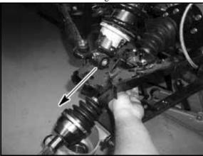
4. Inspect the axle splines and CV boots for any damage.
