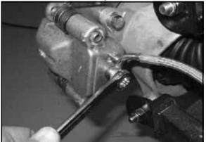
3. After the fluid has drained into the container, remove the two caliper mounting bolts and remove caliper.
