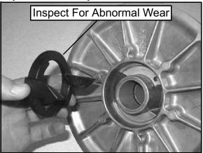
6. Check the rollers in the stationary sheave for wear. If the rollers are worn, a new driven clutch assembly may be needed.
