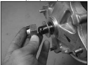
6. Slide the rear hub from the rear drive axle.
