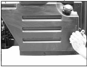
7. Remove the two inner bolts that hold the fuel tank to the frame.
