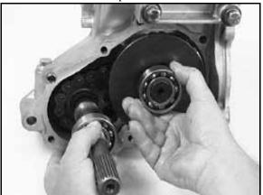
Before installing the cover make sure the sealing surfaces are clean and dry, and shafts are fully seated in the transmission case. Apply Polaris Crankcase Sealant to the mating surfaces.
