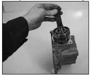
3. Replace the pinion shaft cover O-ring and install the cover. Install the four pinion shaft cover bolts and torque the bolts to 26 ft. lbs. (35 Nm).
