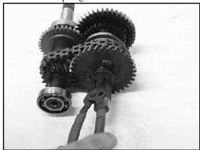
19. Remove low gear (33T) and the needle bearing.
