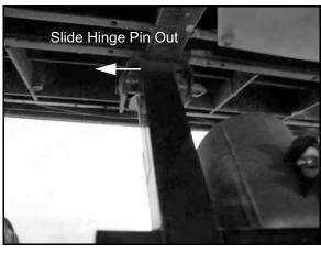
With both hinge pins removed, remove the box from the frame. Two people maybe needed to remove the box from the frame.
