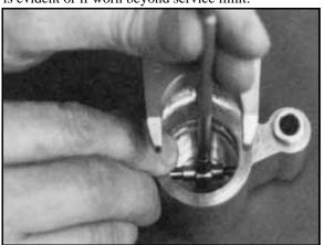
Front Caliper Piston Bore I.D.
