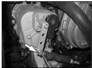
6. Loosen the jam nuts for the transmission cable. Remove the cable from the mounting bracket.
