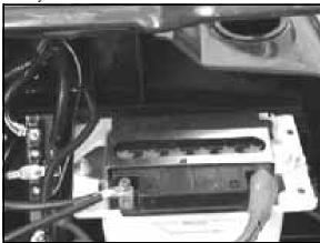
Inspect the battery fluid level. When the battery fluid nears the lower level, remove the battery and fill with distilled water only to the upper level line. To remove the battery:
