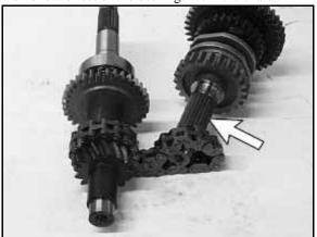
22. Use a press to remove the gear from the shaft.
