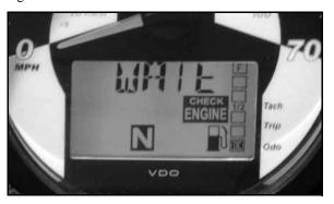
5. Any blink code numbers stored in the EFI module will display, one at a time, on the screen.
