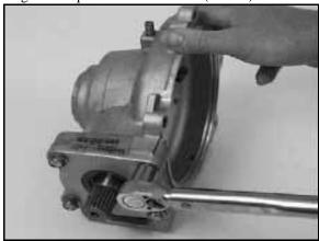
Input Cover Bolts Torque: 17 ft. lbs. (23 Nm)
