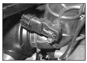
Air passing through the intake is measured by the T-BAP and relayed to the ECU. These signals, comprised of separate air temperature and barometric air pressure readings, are processed by the ECU and compared to it's programming for determining the fuel and ignition requirements during operation.
