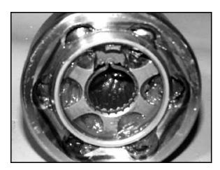
7. Before you assemble the CV joint, slide the new boot (small end first) and clamp over the splined shaft.
