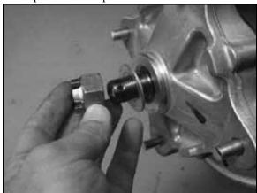
Rear Hub Nut Torque: 110 ft. lbs. (149 Nm)
