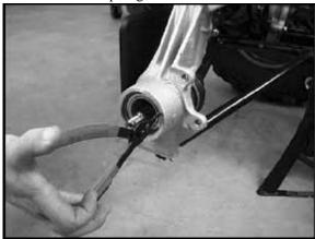
2. From the back side, tap on the outer bearing race with a drift punch in the reliefs as shown in Step 3.
