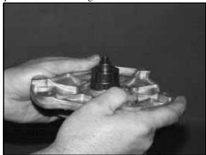
5. Remove nut from puller rod and take installation tool and clutch cover off the rod.
