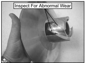
5. Remove the inner spring retainer from the inner sheave. Inspect for wear and replace as needed.
