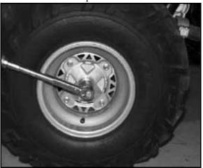
Rear Hub Nut Torque 110 ft. lbs. (149 Nm)
