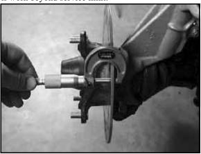
Brake Disc Thickness
