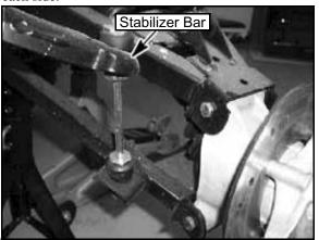
3. Remove the stabilizer bar nut from the lower A-arm on each side.
