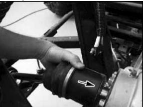
4. Lift bearing carrier into place and install the bolt into the upper control arm. Torque bolt to 30 ft. lbs. (41 Nm).
