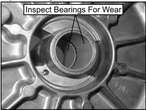
**Moveable Sheave Bearing Inspection:**
