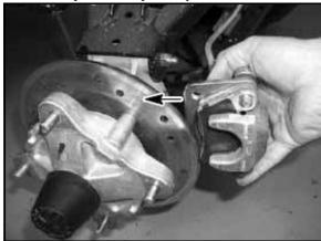
2. Install caliper and torque mounting bolts.
