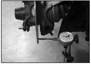
Brake Disc Runout
