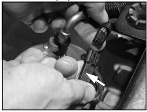
5. Remove the fuel tank vent hose
