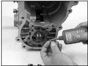
Pinion Retainer Plate Bolt Torque: 6-12 ft. lbs. (8-16 Nm)
