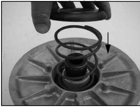
5. Compress the outer retainer and install the snap ring.
