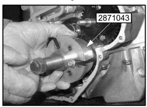
23. Inspect the crankshaft gear (Q) for broken or worn teeth. If the crankshaft gear does not need to be replaced, it does not need to be removed. If the crankshaft gear is damaged, remove the crankshaft gear with the Flywheel Puller (PN 2871043).
