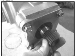
6. If a tight spot is felt during rotation, loosen the backlash screw another 1/8 turn. Perform the previous step again. Repeat this procedure until the pinion shaft rotates smoothly 4 times (1 revolution of ring gear).
