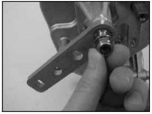
3. Remove the five bolts that secure the cover and remove the cover from the transmission.
