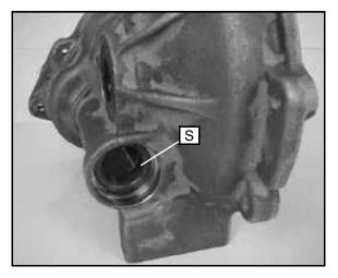
15. Replace all O-ring, seals, and worn components. Replace the seals as shown in the photo.
