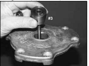
3. With inside of cover toward vise, slide cover onto puller.
