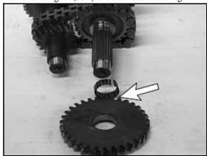
20. Remove the reverse gear shaft.
