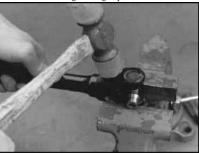
4. Force U-joint cross to one side and lift out of inner yoke.
