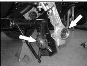
9. With short sharp jerks, remove drive shaft from front gearcase.
