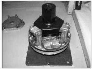
Clutch Holding Fixture: (PN 2871358) Spider Removal Tool: (PN 2870341)
