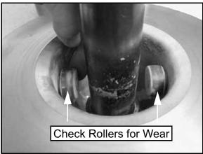
7. Inspect the bearings inside the moveable sheave.
