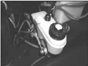
3. If changing fluid, remove old fluid from reservoir with a Mity Vac<sup>TM</sup> pump or similar tool.
