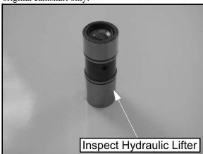
NOTE: Lifters that are scored, worn, or if the bottom is not smooth should be replaced with new lifters and cam as an assembly. If replacing the lifters, the camshaft should also be replaced.
