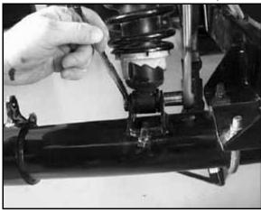
8. Remove the two bolts that secure the rear axle housing to the frame.
