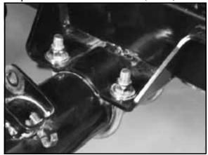
U-Bolt Nut Torque: 40 ft. lbs. (54 Nm)
