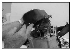
Rocker Cover Bolt Torque:  $84 \pm 8$  in.lbs.  $(9.5 \pm 0.9 \text{ Nm})$ Torque in Sequence 11. Install thermostat (J), new O-ring, and thermostat housing. Torque to specification.
