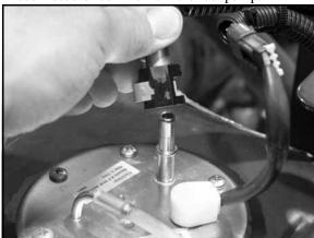
4. Disconnect the fuel pump electrical harness.
