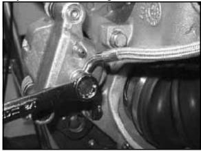
4. Remove brake caliper mounting bolts and caliper.
