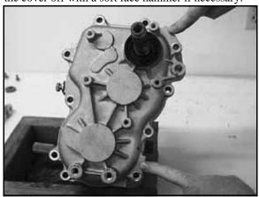
10. Lift shift rail 0.5"-1" (12.70-25.40 mm). Then rotate the shift rail / forks and shift drum, so the forks' pins disengage from the drum.
