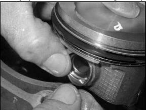
NOTE: If the pistons are to be reused, reassemble the pistons in the same cylinder and direction from which they were removed.
