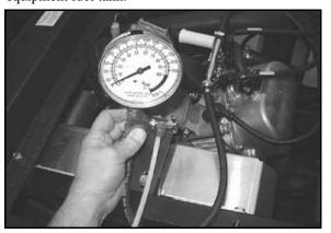
3. Turn on the key switch to activate the pump and check the system pressure on the gauge. If system pressure of 39 psi ± 3 is observed, the ignition switch, ECU, fuel pump, and pressure regulator are working properly. Turn the key switch off and depress the valve button on the tester to relieve the system pressure.
