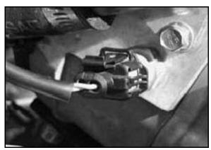
Coolant passes through the cylinder and by the sensor probe, varying a resistance reading which is relayed to the ECU. This signal is processed by the ECU and compared to it's programming for determining the fuel and ignition requirements during operation. The ECU also uses this signal to determine when to activate the fan during operation. If for any reason the engine temperature sensor circuit is interrupted, the fan will default to "ON".
