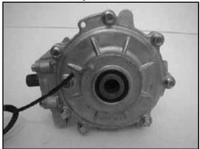
3. Check the gearcase coil resistance. The resistance value should meet the specifications listed below.
