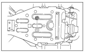
1. Engine oil drain bolt
