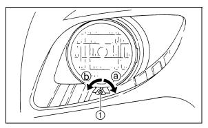
1. Headlight beam adjusting screw
