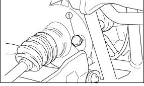
1. Differential gear oil filler bolt
