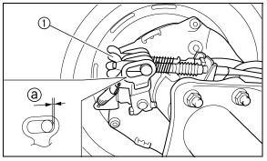
1. Adjusting nut (brake lever cable) a. Gap
