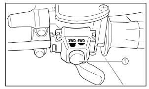
1. On-Command four-wheel drive switch "2WD/4WD"
