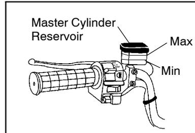
**WARNING:** Once a bottle of brake fluid is opened, use what is necessary and discard the rest. Do not store or use a partial bottle of brake fluid. Brake fluid is hygroscopic, meaning it rapidly absorbs moisture from the air. This causes the boiling temperature of the brake fluid to drop, which can lead to early brake fade and the possibility of serious injury.
