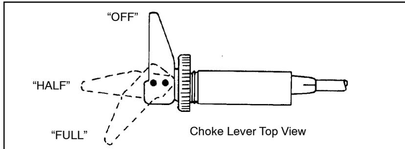
5. Move the choke lever to the FULL position.
