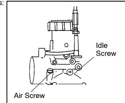
The following variations to air screw adjustment for 2-Cycle engines should be noted:
