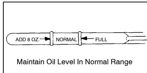
**CAUTION:** Use only Polaris Premium 4 All Season synthetic oil (PN 2871271), or API certified "SH" oil. Never substitute or mix oil brands. Serious engine damage and voiding of warranty can result.
