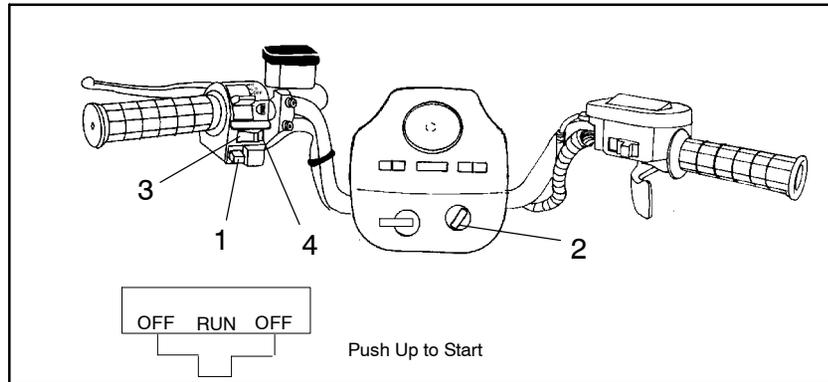
**1. Override Switch (Reverse Speed Limiter)** - This vehicle is equipped with a reverse speed limiter system. To obtain additional power while backing up, depress the override button. **WARNING:** Never activate the override button while throttle is open as loss of control may result, causing severe personal injury or death. **NOTE:** The override switch also allows activation of Demand 4 Drive (All Wheel Drive) in reverse, if Demand 4 Drive switch is on.
