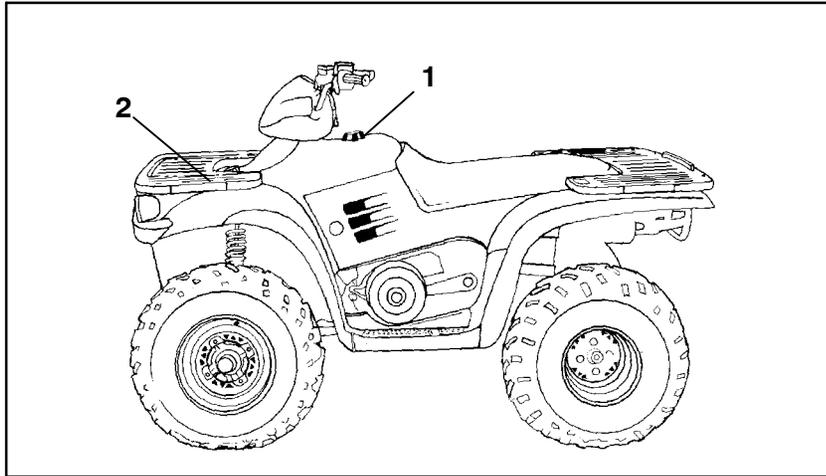
The fuel tank filler cap (1) is located directly behind the handlebar. Refer to your owner's Manual Supplement for tank capacity. Use either leaded or unleaded gasoline with a minimum pump octane number of 87 R+ M/2 octane.
