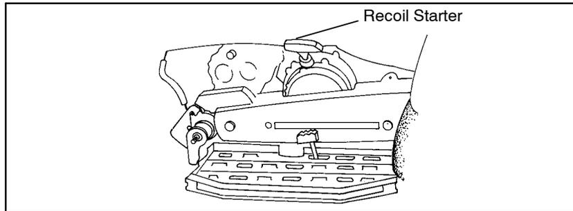
If the battery is weak and cannot start the engine, use of the recoil starter located on the right side of the machine will allow vehicle operation until repairs can be made.
