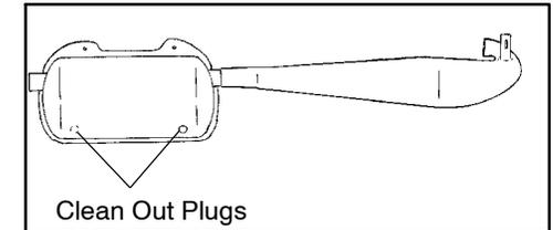
4. If particles are still suspected to be in the muffler, back the machine onto an incline so the rear of the machine is one foot higher than the front. Set the parking brake and block the wheels. Make sure the machine is in neutral and repeat steps 2 and 3. **WARNING:** SEE BELOW.
