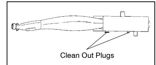
2. Place the transmission in neutral and start the engine. Purge accumulated carbon from the system by momentarily revving the engine several times.
