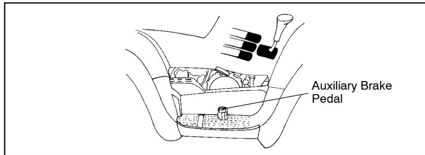
Your Polaris ATV has an auxiliary brake provided as a safety feature. It is located on the inside of the right floor board and is operated by the right foot. It is intended as a backup to the main brake system, especially if the main system becomes inoperative.
