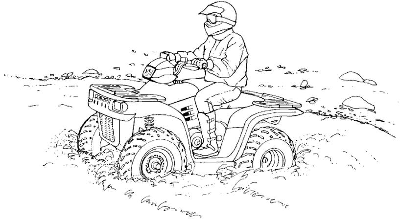
**Your Polaris ATV can operate through water up to depths reaching the footrests. Before fording streams always:**
