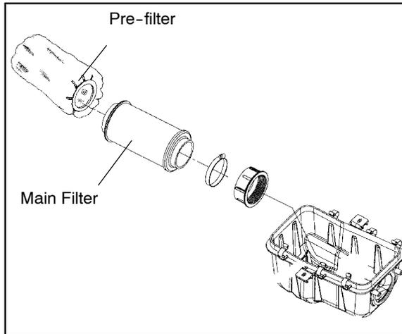
**CAUTION:** Operation of your ATV without a breather filter can cause engine damage.
