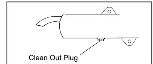
5. If particles are still suspected to be in the muffler, drive the machine onto the incline so the front of the machine is one foot higher than the rear. Set the parking brake and block the wheels. Make sure the machine is in neutral and repeat steps 2 and 3. **WARNING:** SEE BELOW.
