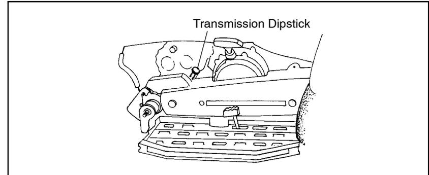
For most models, transmission dipstick is located on the right side of the machine. On the Sportsman, the dipstick is located near the rear brake disc.
